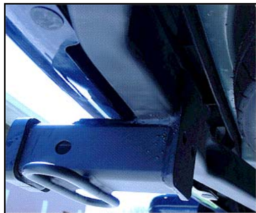
The hitch is now bolted to the frame. Notice how the hitch barely peaks out behind the bumper.
