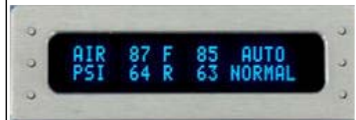
The Slick digital control unit of the ARC-1000
