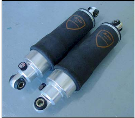
AirRide Technologies SKW7001 Shockwaves. Compressed height of 10.50" and extended height of 14.25"
