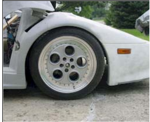
"Slammed" This is the lowest position of the shocks. We would not recommend driving it this low but you can see just how low it can go. It is high enough to clear the fiberglass and not cause any damage in case of an unexpected air pressur loss.
