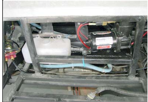
The Air compressor and tank peaking out from behind the dash.
