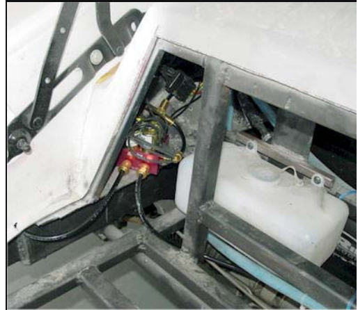
The electric air valves. These control the ride height from switch control in the cockpit.
