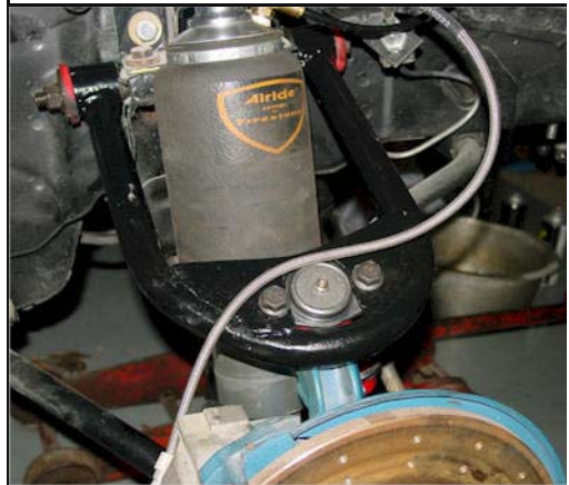
The Shockwaves installed in the old "Coilover's" location with the new A-arms
