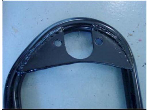
Note the small amount of material behind the ball joint mounting hole. This modified Arm's plate is much thicker than the original providing extra support for the missing material.
